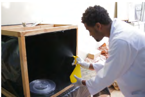
Fig. 11: Showering the chamber with water after inoculation.
